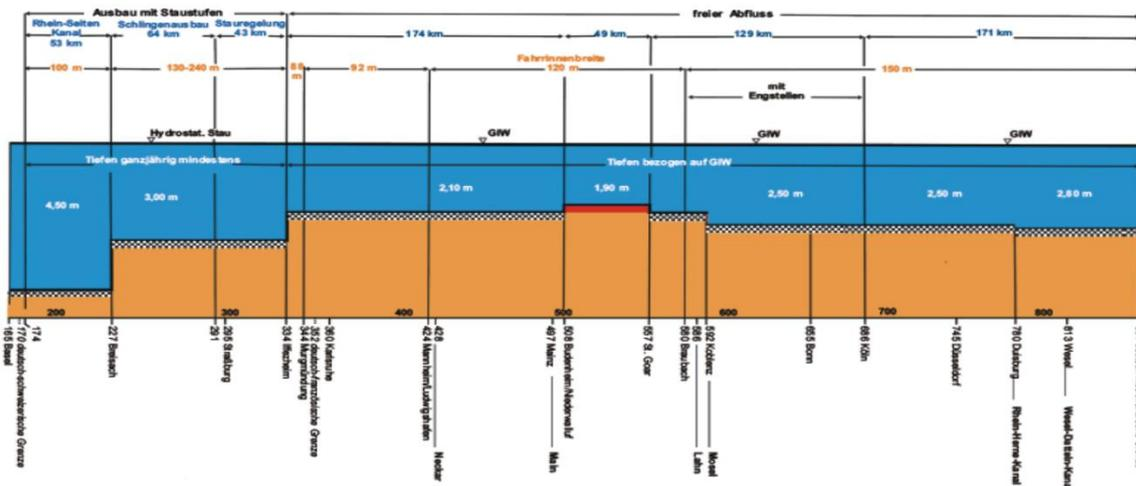
Figure 2: Longitudinal section of the Rhine (Source: WSV)
