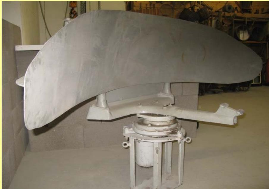
Parabolantenne DECCA Radar 214
