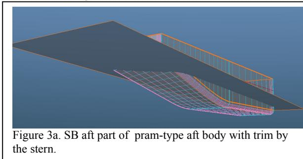
Figure 3a. SB aft part of pram-type aft body with trim by the stern.
