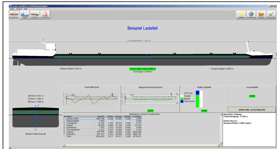
Figure 4. Main screen of LOCOPIAS loading computer of IWW tanker.
