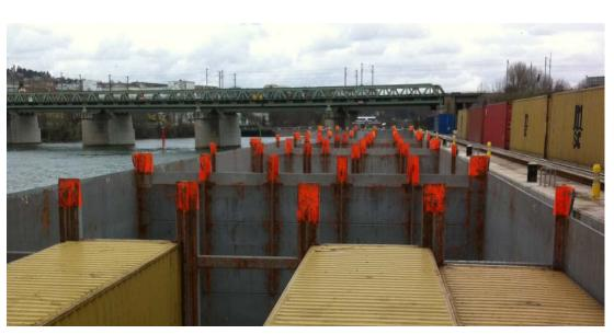
**21.** Container vessels are often loaded with a considerable gap between container rows. This applies, for example, to vessels that are not quite capable of accommodating three rows of containers side-by-side. Please note, however, that if the gap is too big, the containers can shift in the event of heeling, shocks or collisions. Where appropriate, ensure there is no gap between containers.
