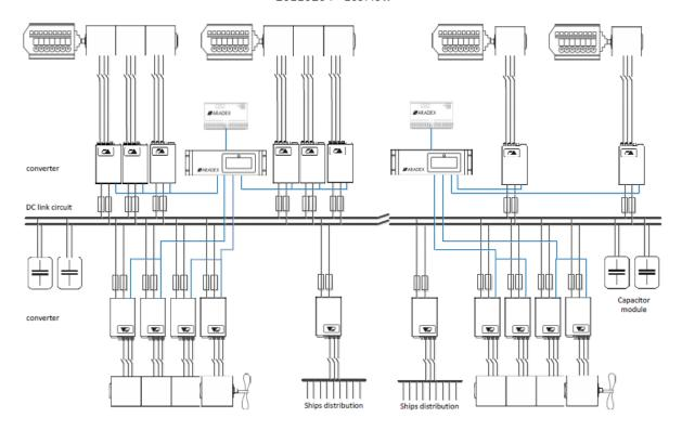
➤ 2 GENSETS with 630 KWe Generator - 3 wather cooled converter eatch With Highspeed Diesel Mitsubishi for 630 KWe bei 1800 RPM
